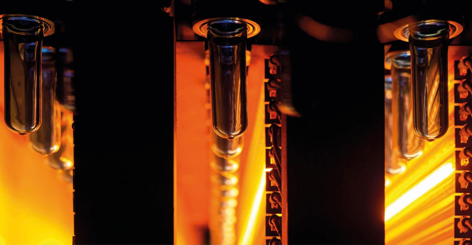
Infrared temperature sensors are helping to provide consistent product quality in the high-speed process of injection blow moulding.
