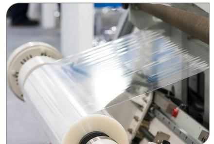
Transmissive materials are difficult to measure. A specialised sensor such as the PyroCube P may be required to achieve a good reading.
